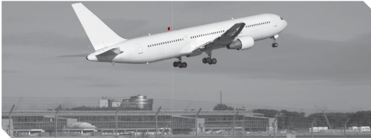
The aeroplane has engines that provide applied force that enables the aeroplane to move forward. Air resistance acts in the opposite direction of movement of the aeroplane. Gravity acts downwards on the aeroplane, while an upward force on the wings of the aeroplane help it to move upwards. As the applied force and upward force are greater than the forces acting on them (air resistance and gravity), this helps the plane fly and stay in the air
