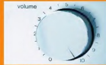
▲ Figure 8.1 Turning this dial alters the resistance in the circuit which changes the volume of the sound.
