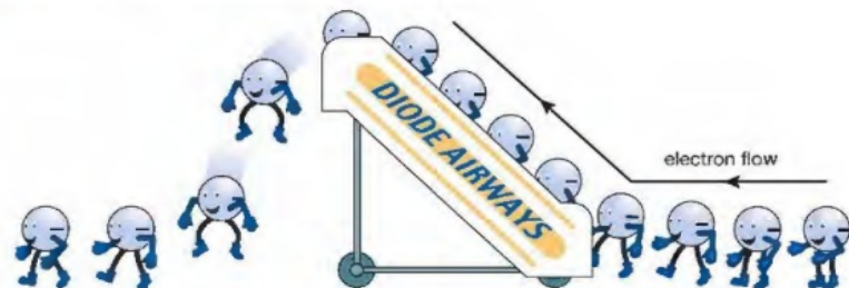
▲ Figure 8.17 Diodes will only let charges flow one way.
