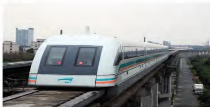
▲ Figure 8.20 Maglev trains use superconducting magnets to help them hover above the tracks.
