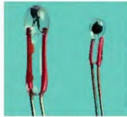
▲ Figure 8.14 Two examples of thermistors and their symbol – the resistance of a thermistor changes a lot as the temperature changes.
