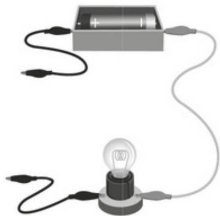
6 Attach the alligator clips to the fasteners.
