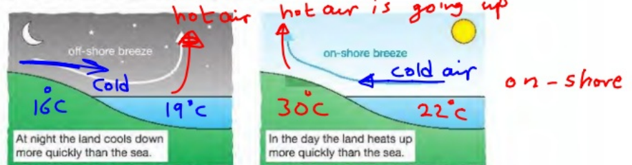
▲ Figure 15.8 At night the air over the warmer sea floats up causing cooler air to flow towards sea.
