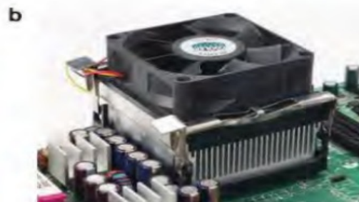
▲ Figure 15.13 a A shiny kettle stays warmer longer. b The heat sink needs to be matt black to lose heat to the surroundings quickly, and so stop the transistor overheating.
