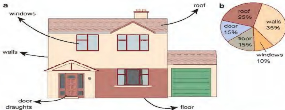
▲ Figure 15.18 a How heat energy can be lost from the home; b Percentage of energy lost in different ways
