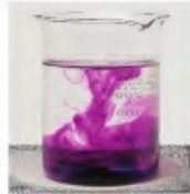
▲ Figure 15.4 Demonstration of convection currents, using a potassium manganate (VII) crystal in water
