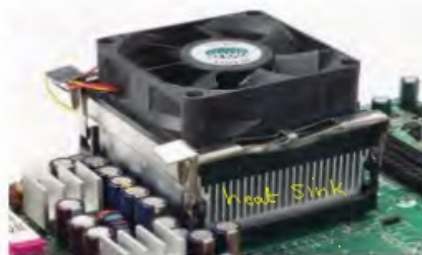
▲ Figure 15.13 a A shiny kettle stays warmer longer. b The heat sink needs to be matt black to lose heat to the surroundings quickly, and so stop the transistor overheating.
