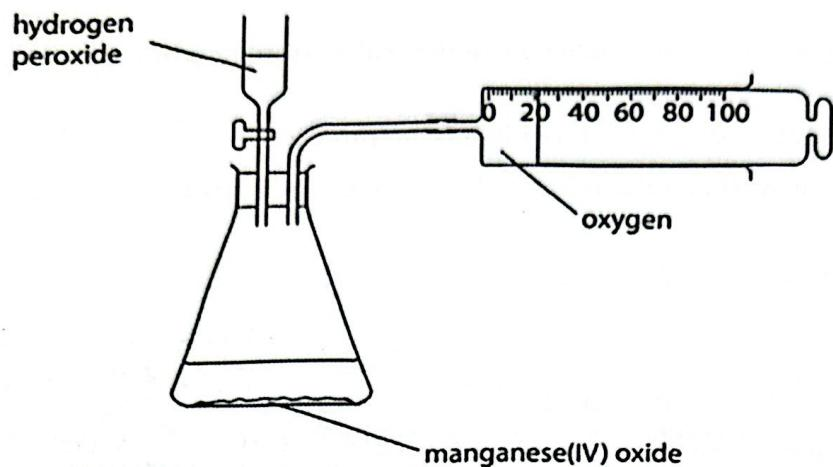
(a) Describe a test to show that the gas collected in the syringe is oxygen.
