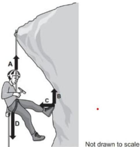
a) Which arrows A, B, C, or D represents the force of gravity acting on Ryan? **D**
