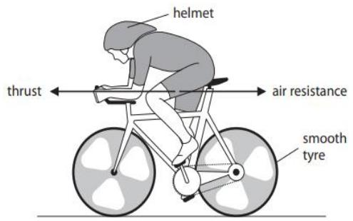
The cyclist will speed up, because thrust is greater than air resistance. The greater force is acting into the direction of movement
